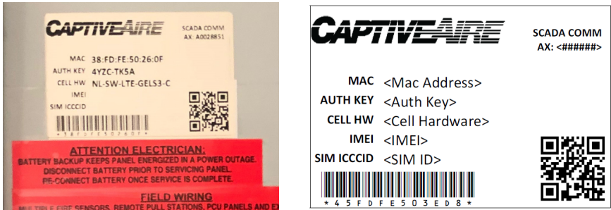
Figure 10 - The Auth. Key and MAC Address Locations
