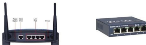
Figure 6 - Wireless Router/Ethernet Switch
